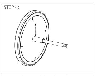
Using an allen wrench, loosely install set screw. Set screw should align with notch in axle. \*Do not fully tighten set screw until STEP 6.
