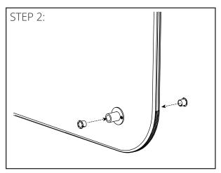
Insert plastic bushings into both sides of panel.
