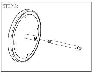
Insert axle into wheel assembly. Ensure axle is fully inserted into wheel assembly.
