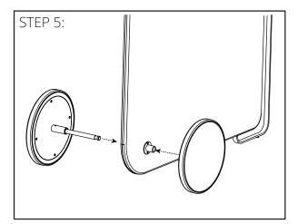
Slide axle through panel and into opposite wheel assembly. Push both wheel assemblies tight against panel.
