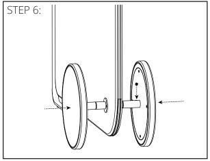
While pushing inward on both wheels, install set screw into second wheel assembly. Set screw should align with notch in axle. Give both set screws a final hand tighten.
