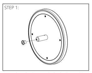
Insert plastic bushing into both wheel assemblies.
